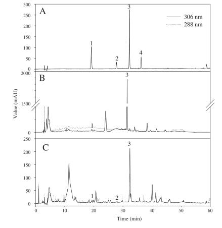
Fig. 1. HPLC chromatogram of standards (A), 'Beiquan' berry skins (B) and leaves (C) after UV-C irradiation at 306 nm (solid line) and 288 nm (dotted line). The numbers 1–4 in the chromatogram indicate *trans*-piceid, *cis*-piceid, *trans*-resveratrol and *cis*-resveratrol, respectively.
